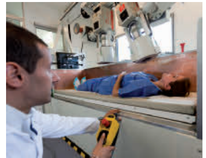
Radiological control of thyroid (top) and whole body counting (above) are performed on supposedly exposed individuals.
