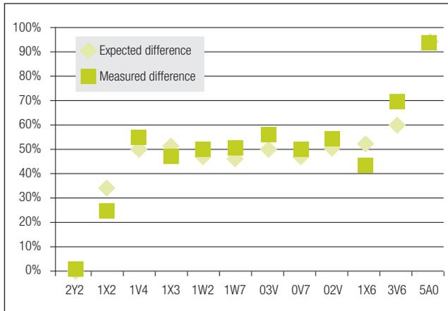
Figure 2 Expected and measured intensities relative to PWR assembly 2Y2
