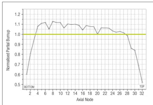
Figure 1 Example for a typical axial burnup profile for a PWR
