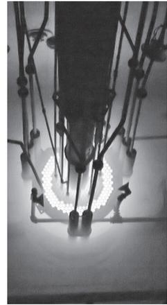
Cherenkov flash during a pulse irradiation in the NSRR
