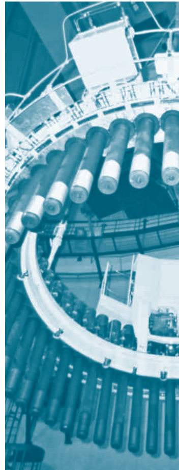
Reactor vessel bolting machine at Penly NPP (France)
