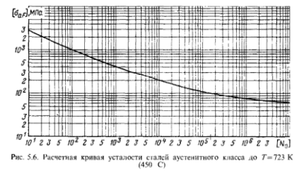
Figure 2: Fatigue curve (dependency of fictitious stress amplitude on number of cycles) for austenitic steel up to 450 °C according to /PNA 86/.
