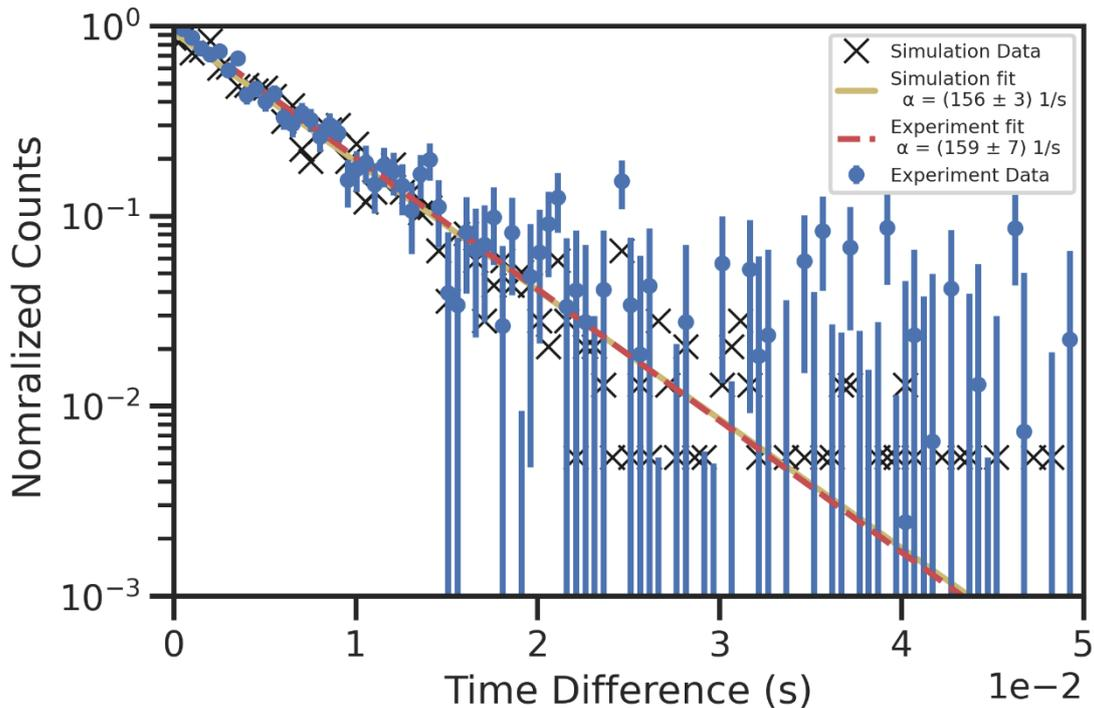
Figure 4 - The blue dots are the experimental points with their respective error bars, the red dashed line is the fitted function of the Rossi- $\alpha$  method to the experimental data points. The black crosses are the points obtained by simulation and the line in yellow is the fitted function of the Rossi- $\alpha$  method. The curves were normalized to represent only the exponential part of equation (1) for better contrast.
