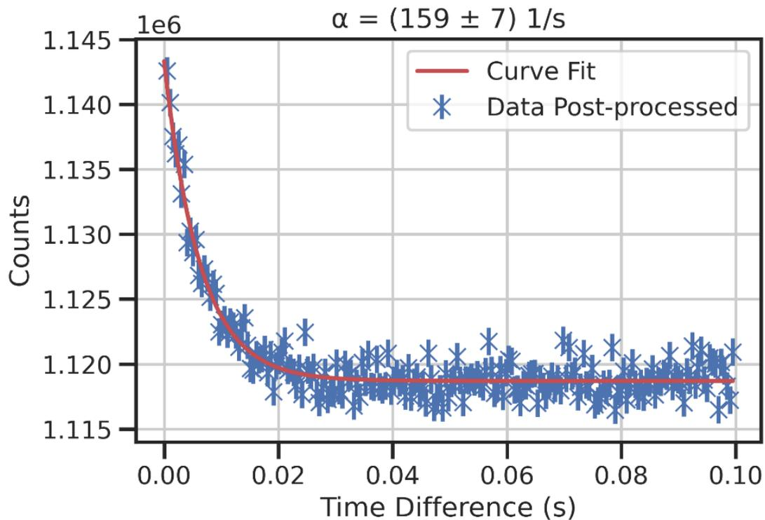
Figure 3 - The time differences are represented by the blue crosses with their associated error bars, the red line corresponds the fit of equation (1) conducted by the non-linear least-squared method.
