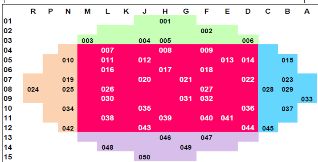
In-core neutron flux and coolant temperature IITA (50 IITA sensors)
