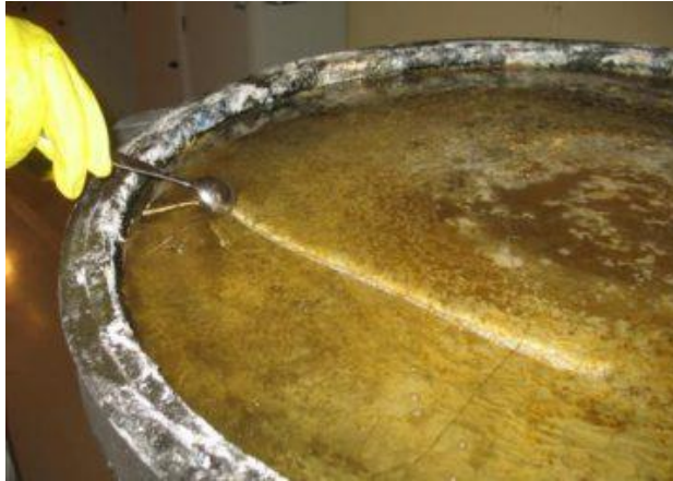
Drum containing a layer of gel on the concrete surface. Taken from https://www.stora.org/fr/node/602
