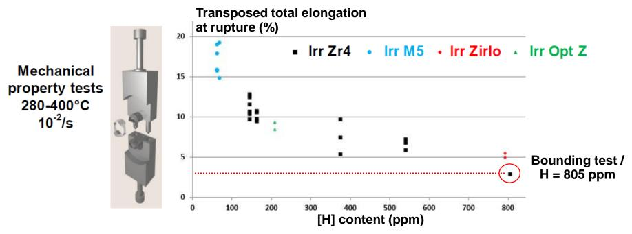
EDF's proposal: the 1% plastic circumferential strain criterion is applicable to PCC-2 power pulse for M5, ZIRLO and Opt ZIRLO
