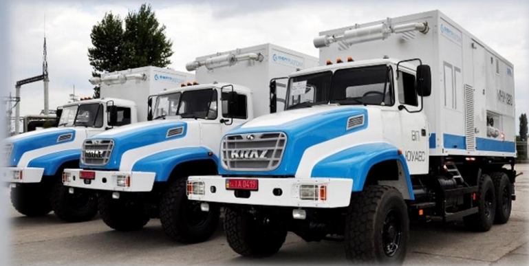
Option 1: mobile diesel-driven pump + 0.4 kV 'small' mobile diesel generator
