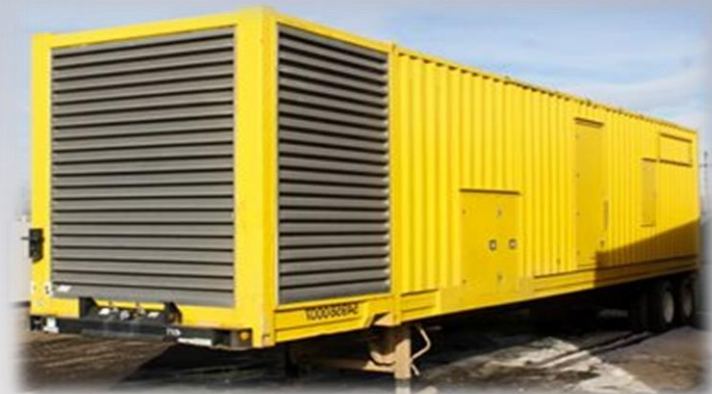
Option 2: 6.3 kV 'big' mobile diesel generator
