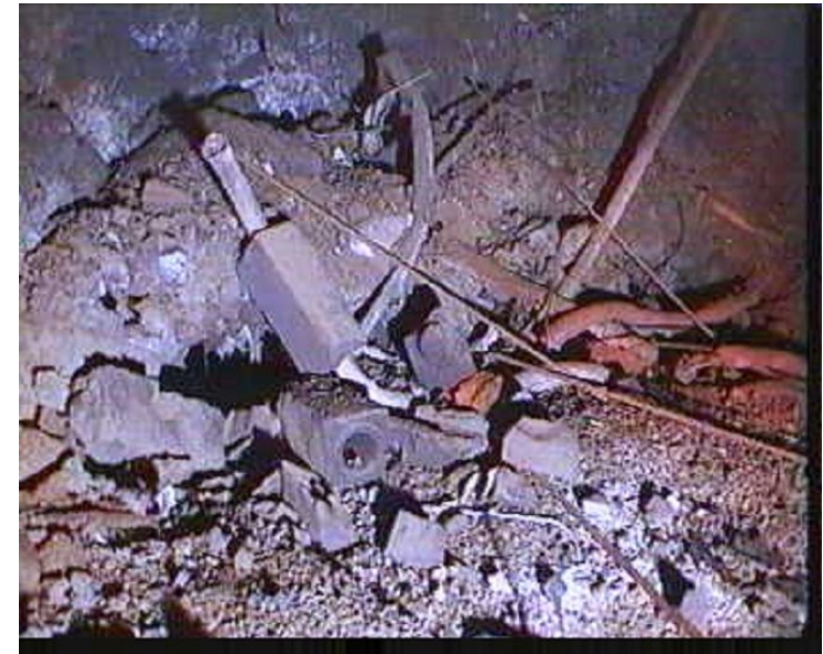
Fuel element fragments, graphite and fuel lava
