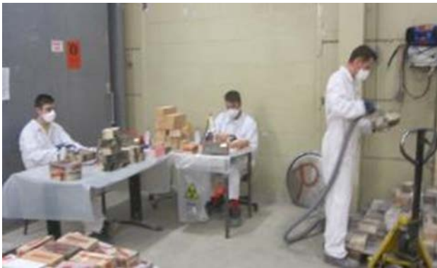
Measurement of contaminated bricks
