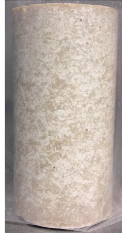
Matrix of magnesium oxide with crushed salt inclusions, produced in GRS laboratory
