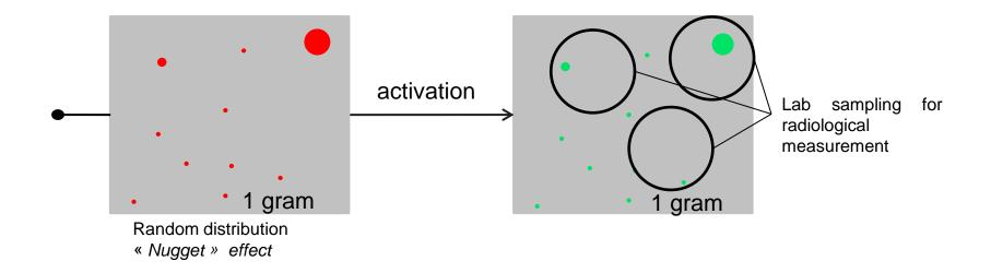
For many radionuclides, radiological measurements exhibit high discrepancies (2-3 orders of magnitude) that do not correlate with the neutron flux variation (1 order of magnitude), or the temperature variation (280-530°C)
