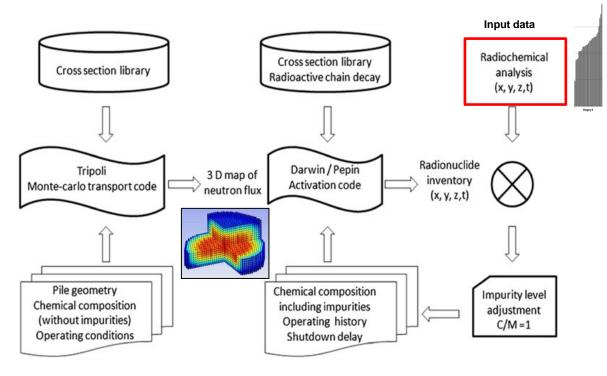
For each of the j local measures  $M_{ij}(x_j, y_j, z_j, t_j)$  of a radionuclide i, a local activation matrix  $A_j$  is analytically built using the calculated local neutron flux.
