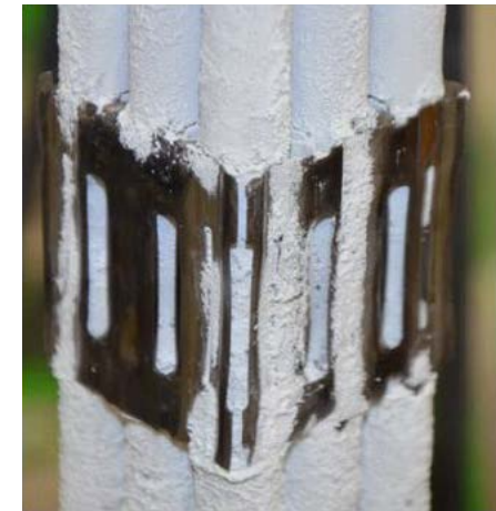
Source: Report HZG-IPM-1501431 Deposition at bundle spacer (Test RLII-HZ9-V13)
