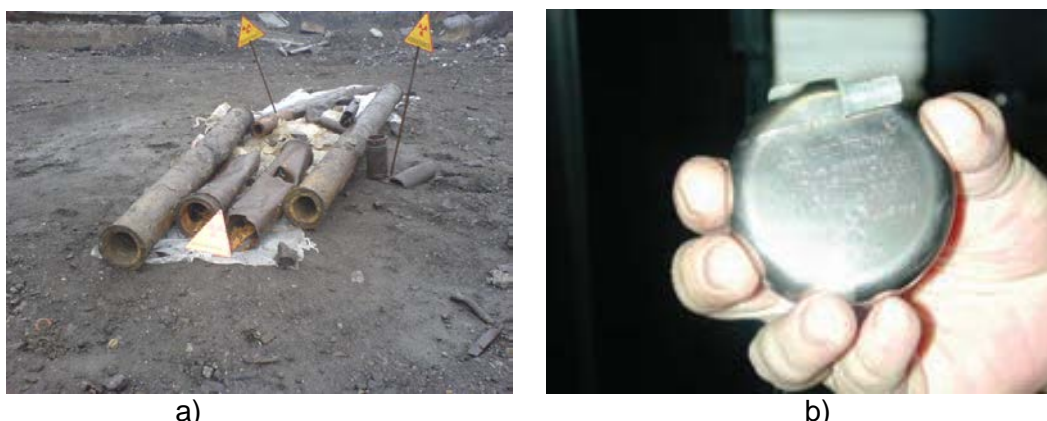
Fig.4. Primary targets of unlawful acquisition of radioactive wastes in Ukraine: a) radioactive contaminated metal scrap, especially nonferrous; b) spent sealed radioactive sources
