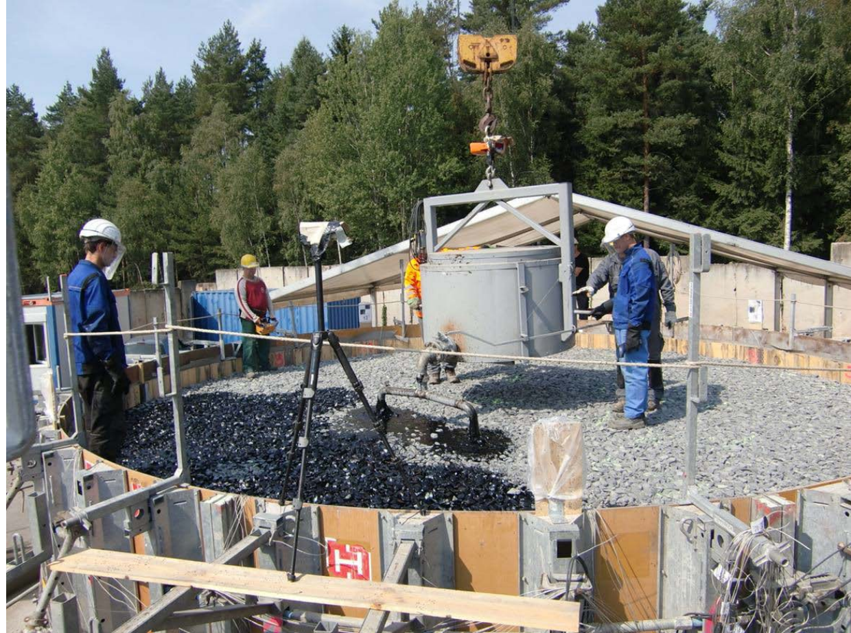
Real scale for shaft sealing elements (diameter: 8 m)
