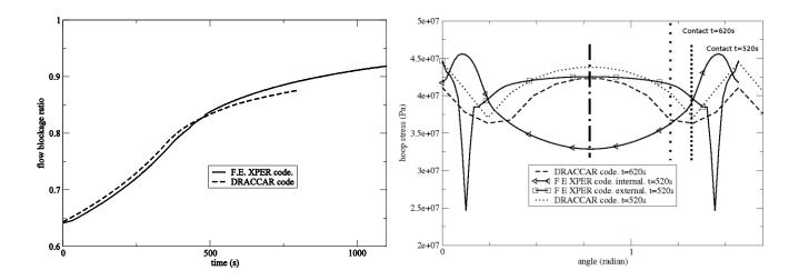
Figure 3. Test-case 3: comparison between DRACCAR and XPER results. On the left : flow blockage ratios evolutions ; on the right : hoop stresses evolutions along one quarter of the cladding perimeter.
