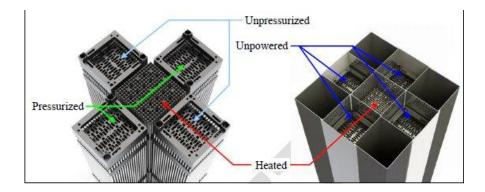
Figure 10. Layout of the Phase II test assembly
