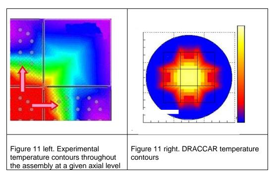
This specific geometry can be modelled using axis-symmetric codes but at the cost of some simplifying hypotheses to reproduce at best average experimental values. However, in order to get some "correct" code results, parametric tunnings are necessary to fit at best the experimental results.
