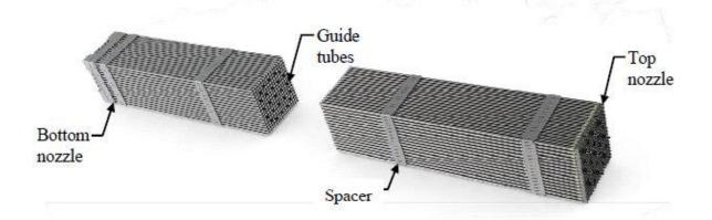
Figure 9. Various components in a typical 17×17 PWR fuel assembly
