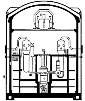
Figure 4: schematic view of a French1300 MWe PWR horizontal floors surrounding the reactor cavity
