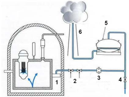
Figure 5: schematic view of the French1300 MWe PWR EFCVS 1 = Metallic prefilter ;
