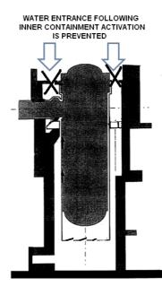
Figure 3: preventing the reactor cavity to be flooded (dry cavity) (schematic view)
