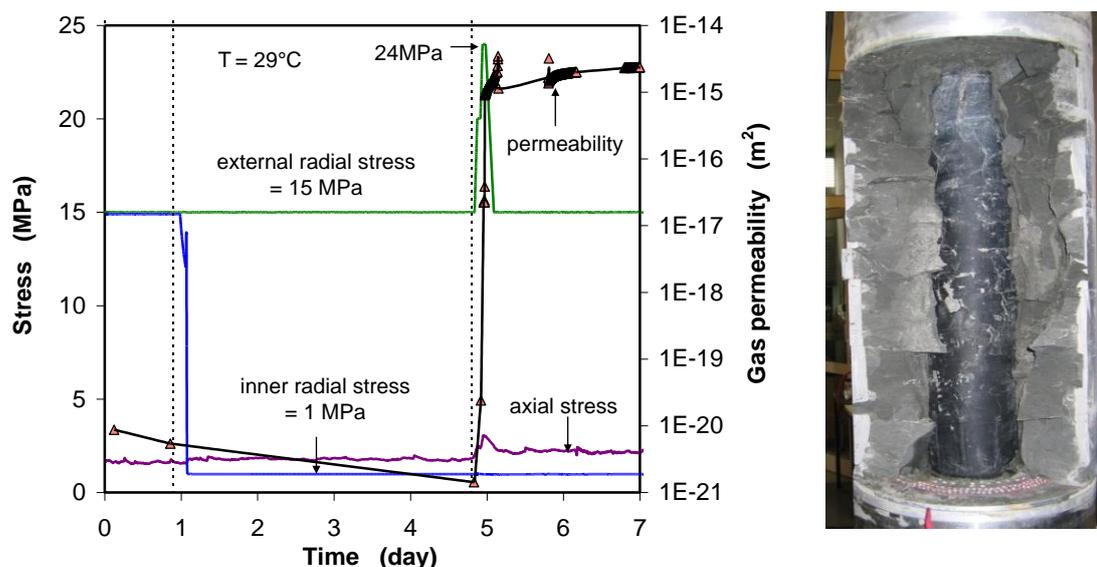
**Fig. 7** Fracturing-induced permeability changes in a large hollow cylinder of COX claystone
