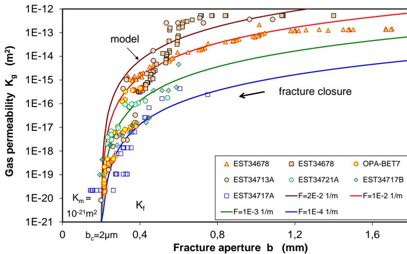
Fig. 2b Fracture permeability – aperture relationship
