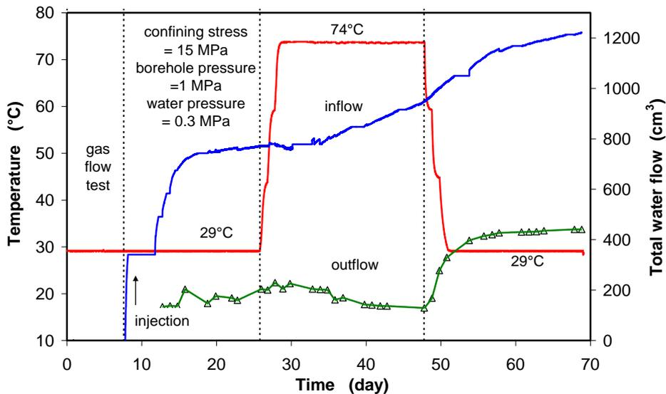
Fig. 9 Water flow through the EDZ in a large hollow cylinder of COX claystone before, during, and after heating
