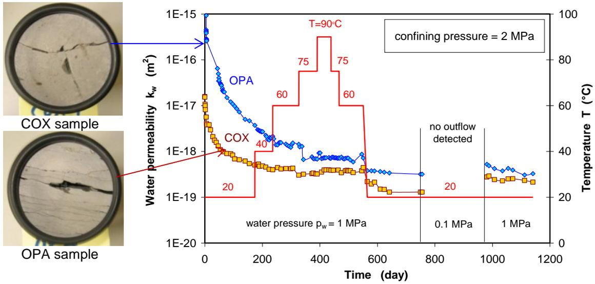
**Fig. 5** Long-term measurements of water permeability on fractured COX and OPA claystones during heating and cooling
