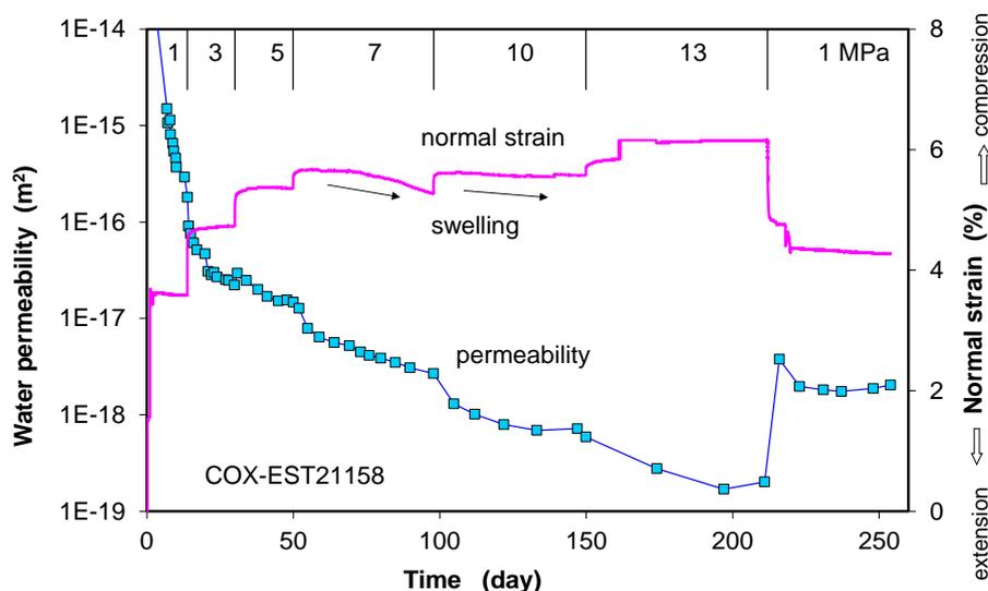
a. normal strain and permeability parallel to fractures during water flowing
