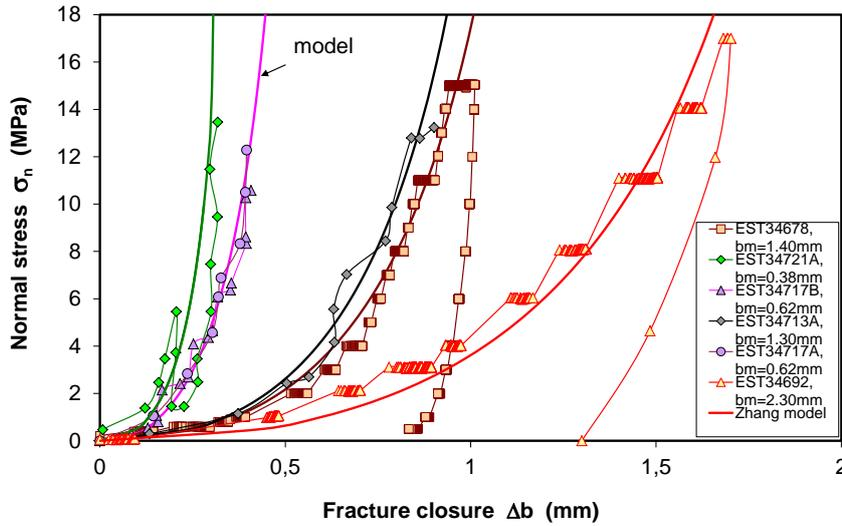
Fig. 2a Fracture closure – normal stress relationship
