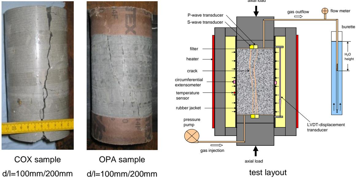
**Fig. 1** Pictures of fractured clay samples and principle of triaxial sealing test
