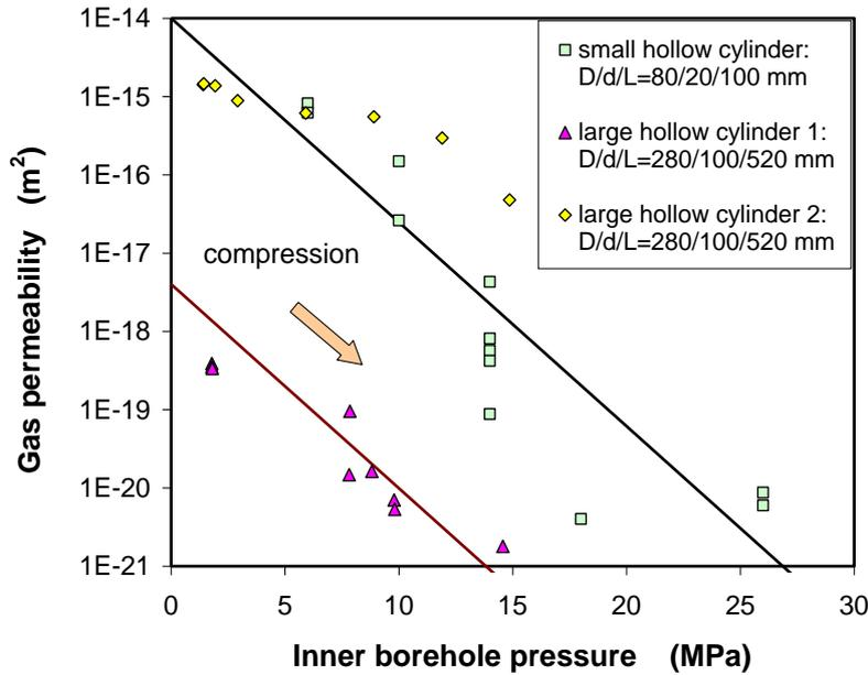
Fig. 8 Compaction-induced permeability decrease in the EDZ around boreholes
