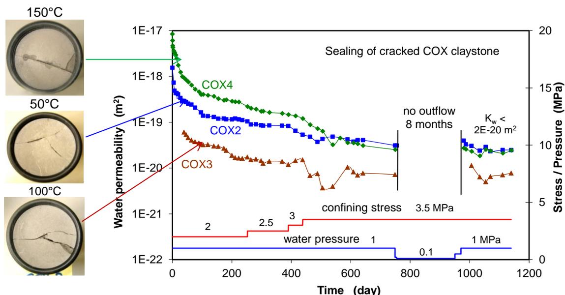
**Fig. 4** Long-term evolution of the water permeability of fractured and pre-heated claystone under different confining stresses
