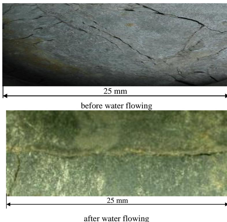
b. fracture patterns before and after water flowing
