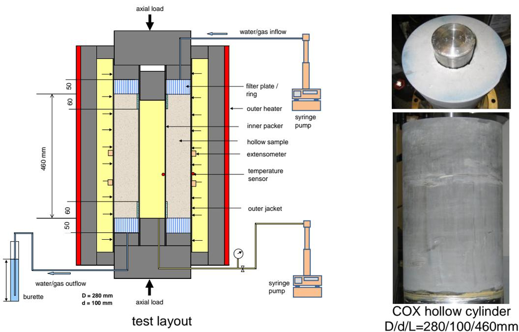
**Fig. 6** Principle of large hollow cylinder tests for investigation of fracturing and sealing of the damaged zone around boreholes under relevant repository conditions
