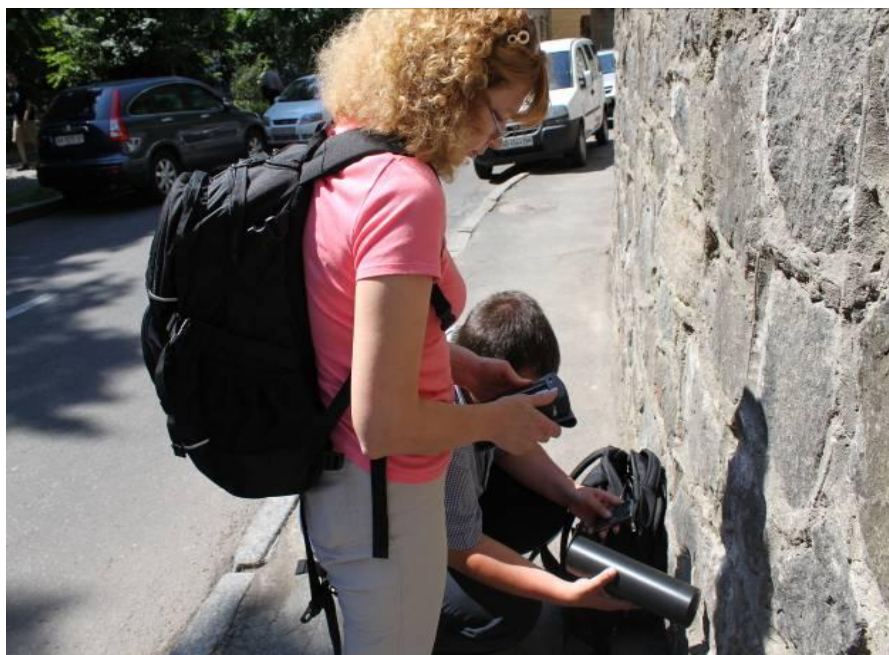
Radiation survey of suspicious spots (dose rate to 2 \mu\text{Sv/h} )
