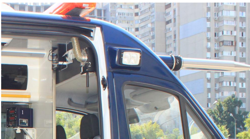
Fig.1.4 – Air sampling system: 1-air collection controller, 2-filter holder, 3-air samplers
