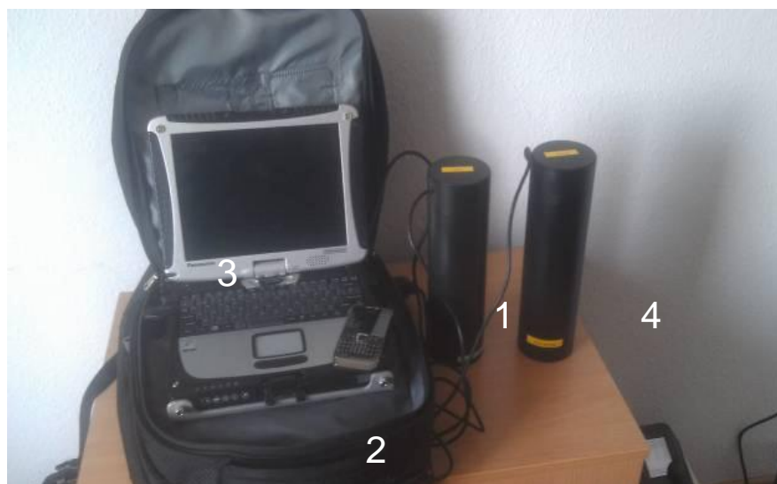
Fig.1.6 – Portable measurement system Vasikka in a backpack. 1 – neutron detector with digital multi-channel analyzer; 2 – remote control palmtop; 3 – laptop with software, GPS-receiver and database; 4 – LaBr gamma with digital multi-channel analyzer
