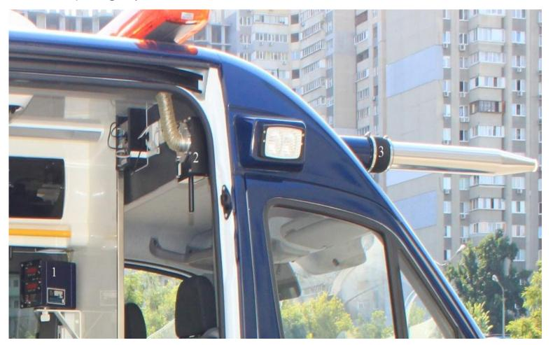
• The RanidSONNI is equipped with a portable spectrometer "ORTEC-AMETEK" on the basis of pure germanium (with electric cooler), what allows making measurements of samples and filters directly at the sampling point.
