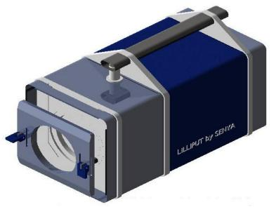
The stand-alone sampler is portable and battery-powered; so they can be dropped at any location for fully autonomous sampling. The filters are laminated into a plastic cassette, which makes sample handling easy. Sample preparation is not needed before measurement because of the design of the filter cassette. Air consumption is up to 12 m<sup>3</sup>/h.
