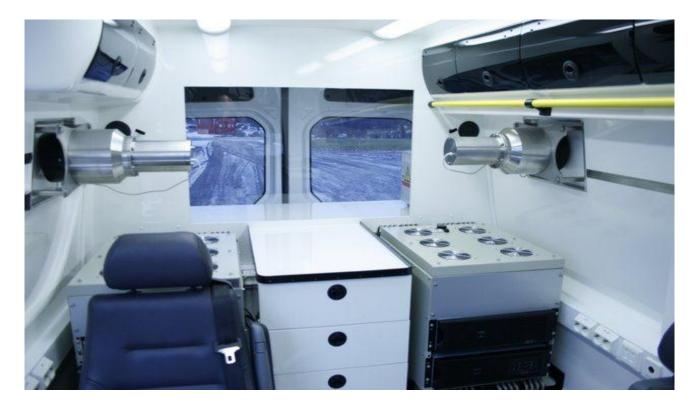
RanidPro100 LaBr3 detector is mounted in front of the vehicle. It is located above and in between the driver and codriver's seats. It is installed inside a 10 mm thick background radiation shield tube opening in the direction of travel. This type of collimation makes it possible to provide a spatial scan of the incident site from a distance.
