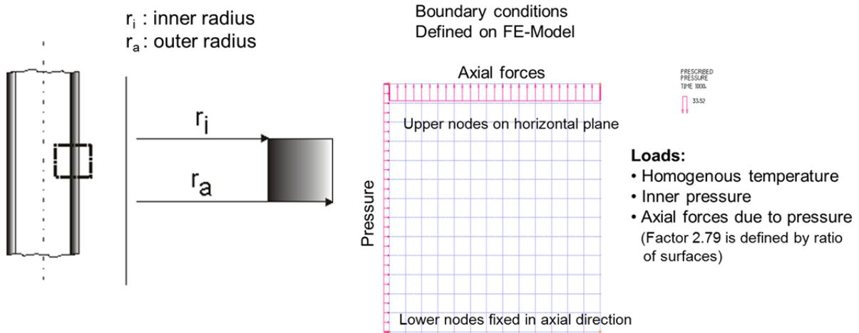
Fig. 12: 2D-Representation of pipe structure, dimensions, loads and boundary conditions
