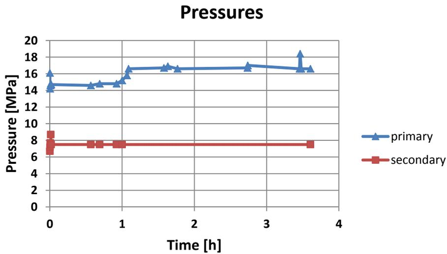
Fig. 2: Pressures versus transient time for primary and secondary circuit positions
