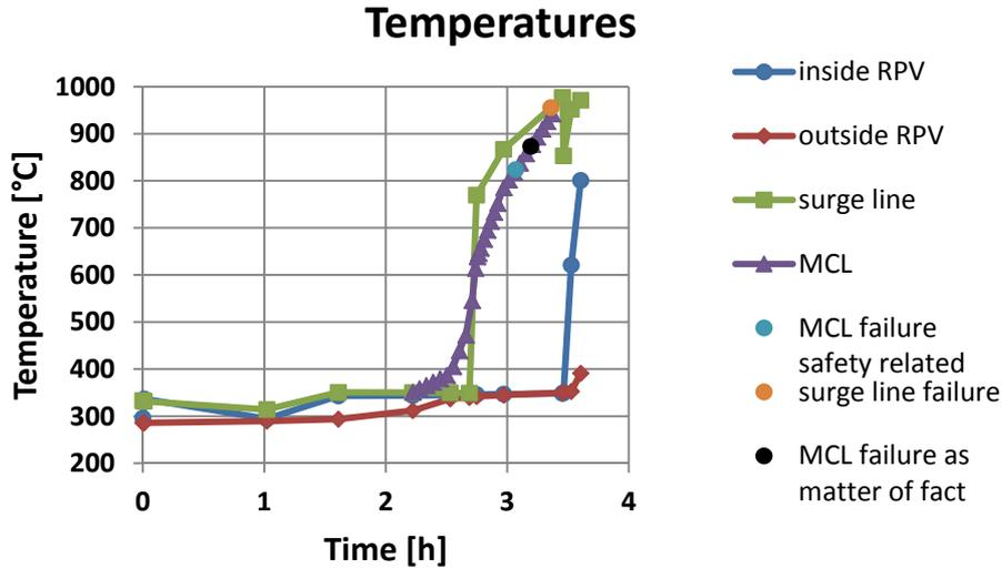
Fig. 6: Temperatures versus transient time for different positions together with times and temperatures of failure for MCL and surge line
