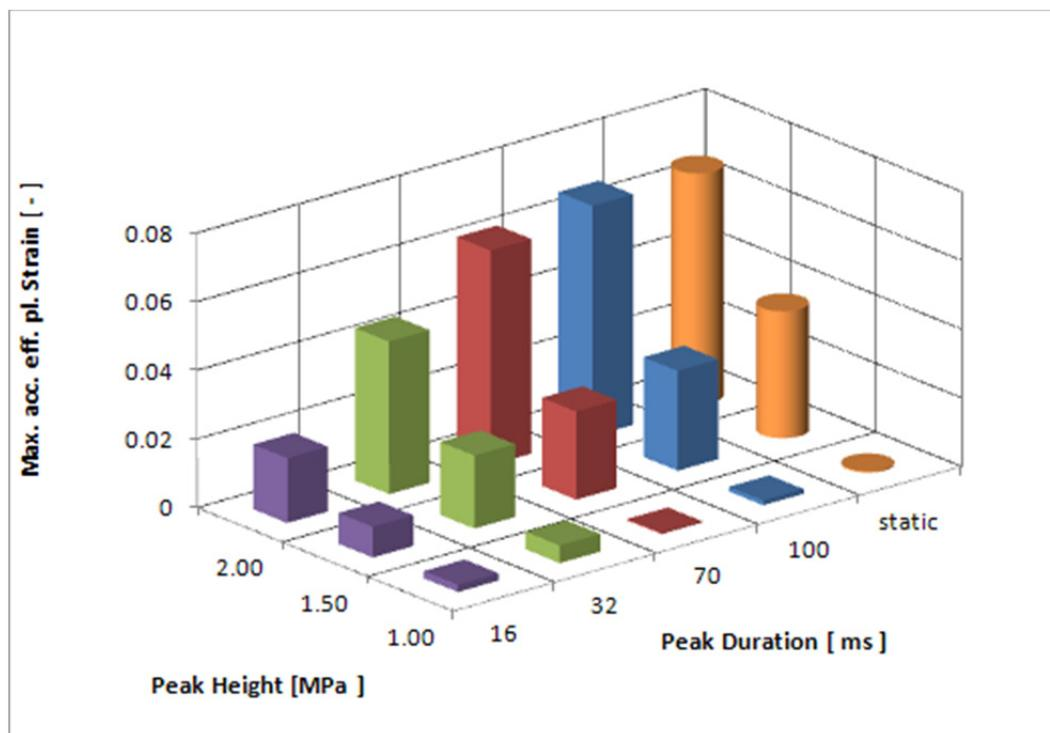
Fig. 24: Maximum values of accumulated effective plastic strain for several peak heights and durations, 3D model with symmetric loading
