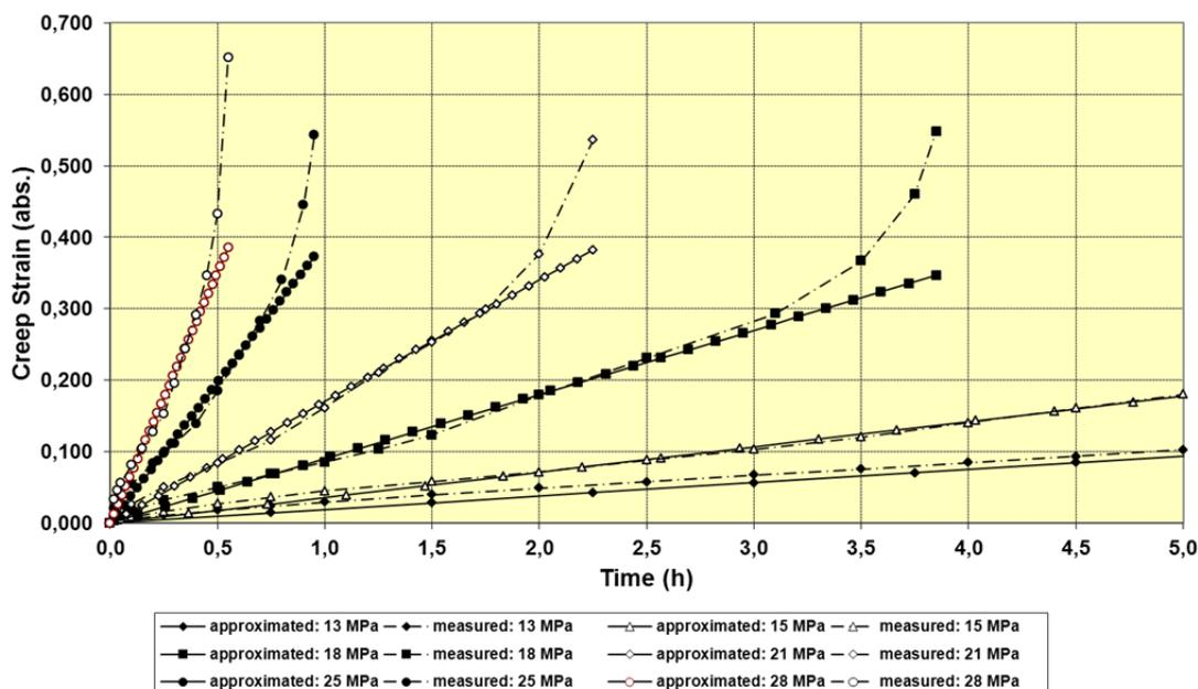
Fig. 10: Linear approximation of measured creep curves (load controlled) of steel 20 MnMoNi 5 5 at 1000°C
