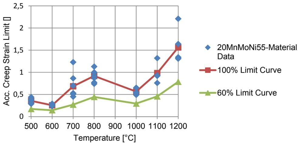
Fig. 11: Steel 20 MnMoNi 55 – Approach for definition of uniaxial creep limit
