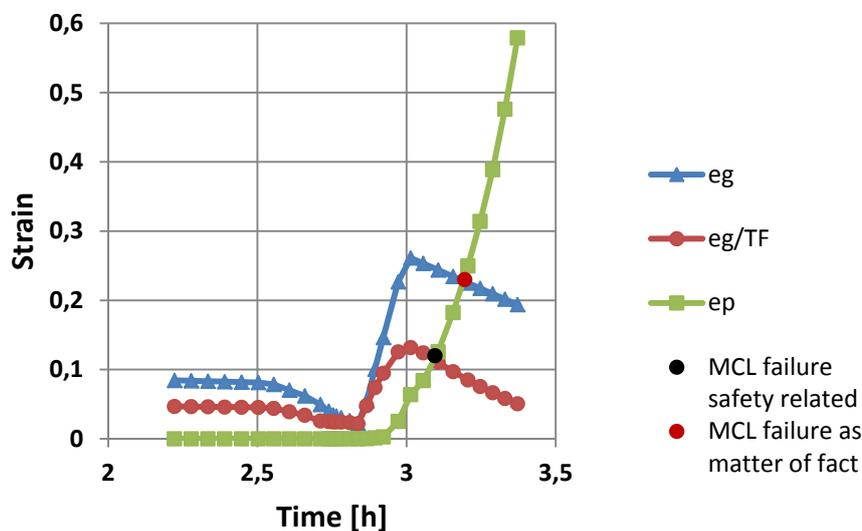
Fig. 4: Integrity assessment for a typical integration point in the MCL
