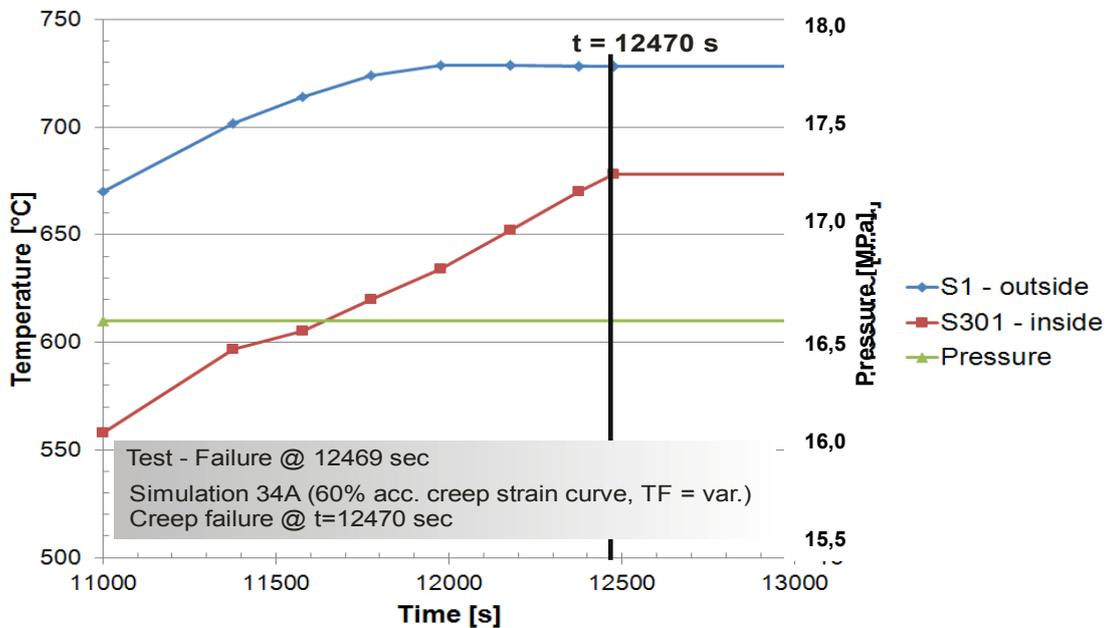
Fig. 14: Loading conditions in the test pipe
