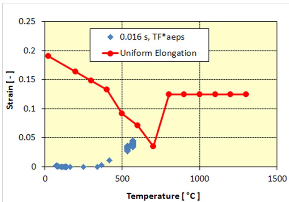
Fig. 25: Calculated strains times triaxiality factor versus temperature for relevant elements of the containment model compared with uniform elongation after 16 ms, case: peak heights 1 MPa and 800°C, peak duration 32 ms
