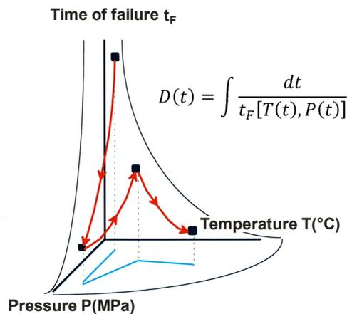
Fig. 8: Linear damage accumulation hypothesis in ASTOR
