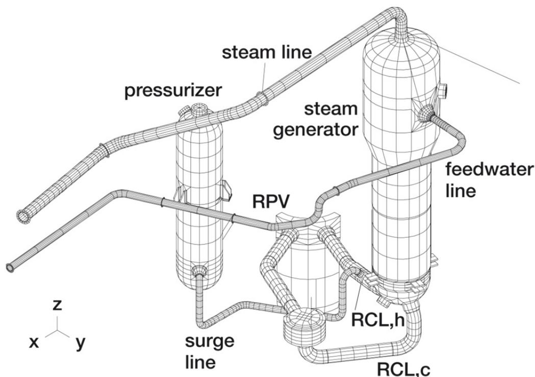
Fig. 3: FE-model of the coolant loop including surge line and pressurizer
