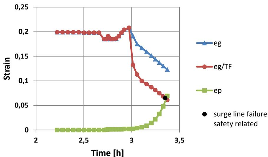
Fig. 5: Integrity assessment for a typical integration point in the surge line
