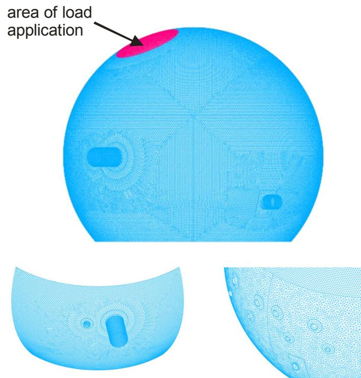
Fig. 21: Finite Element model of the steel containment with penetrations, complete model and parts
