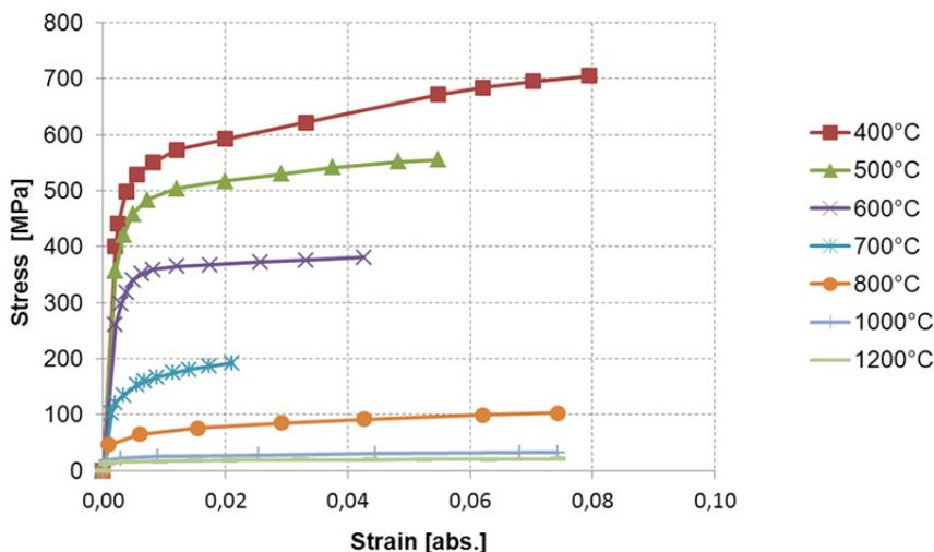
Fig. 9: Steel 20 MnMoNi 5 5: true stress-strain curves up to uniform elongation (400°C – 1200°C) derived from measured data
