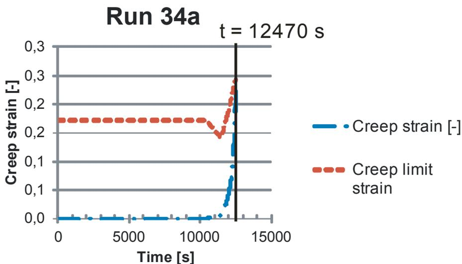
Fig. 15: Accumulated creep strain and strain limit curve (failure at 12470 s)
