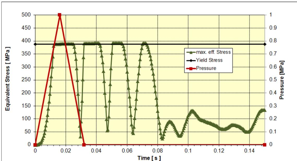
Fig. 23: Time dependency of equivalent stress for the point with the maximum value in comparison to yield stress
