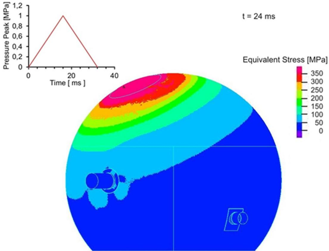
Fig. 22: Distribution of equivalent stresses at t=24 ms
