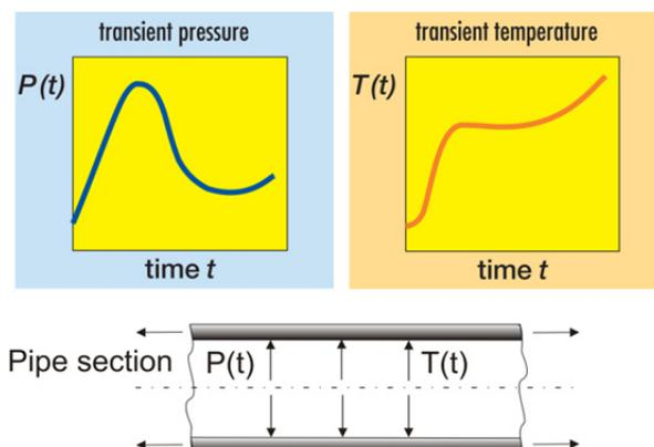
Fig. 7: Transient loads on pipe
