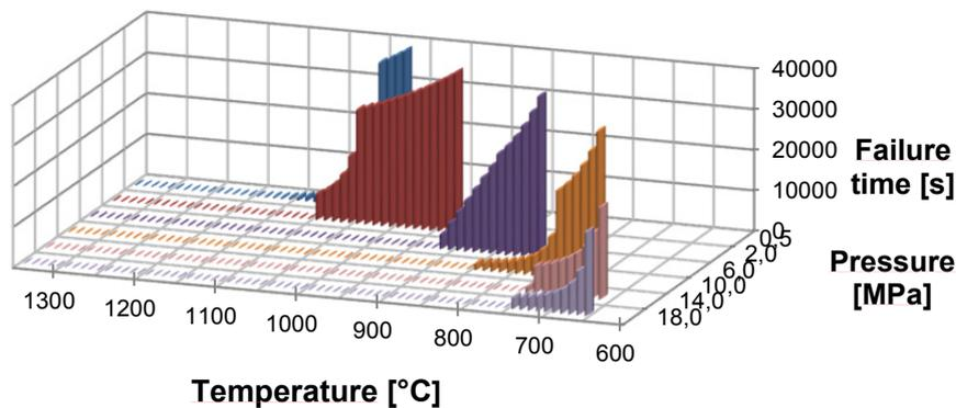
Fig. 13: Failure time diagram for a RCL of 20 MnMoNi 5 5
