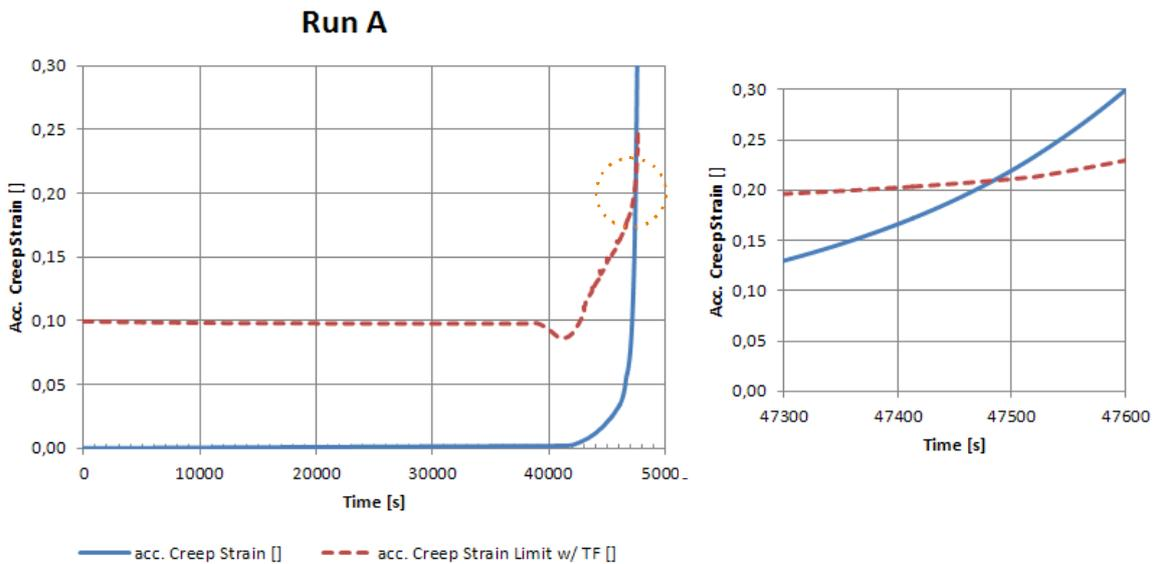
Fig. 17: Accumulated creep strain and strain limit curve (failure at 47471 s), overview and detail view
