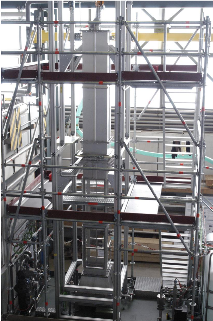
PSI: TRISTAN facility for investigation of two-phase flow characteristics
