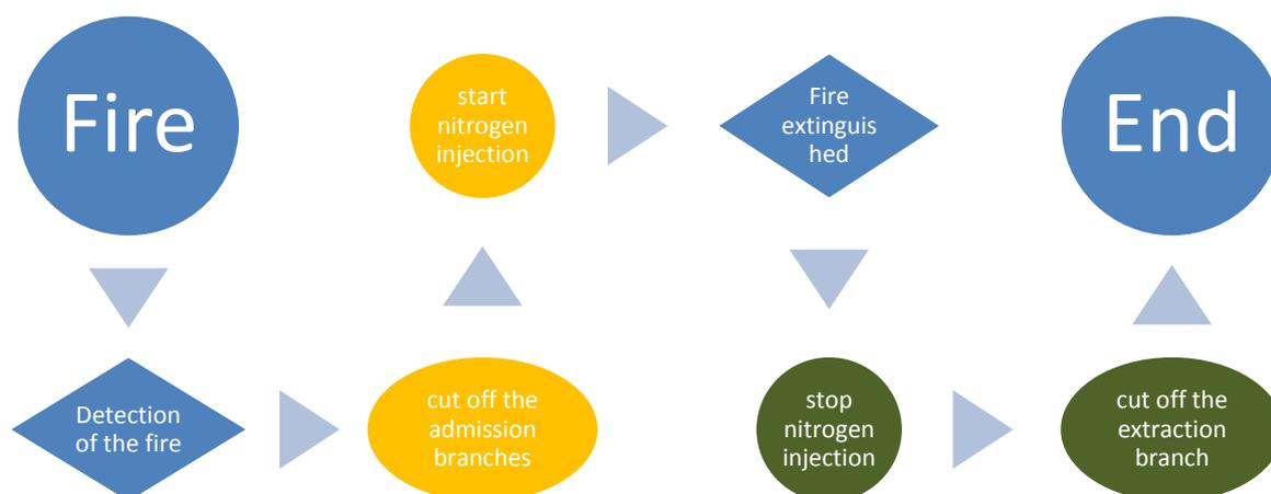
Figure 13: Sequence of control strategy for large single hot cell within the specific facility
