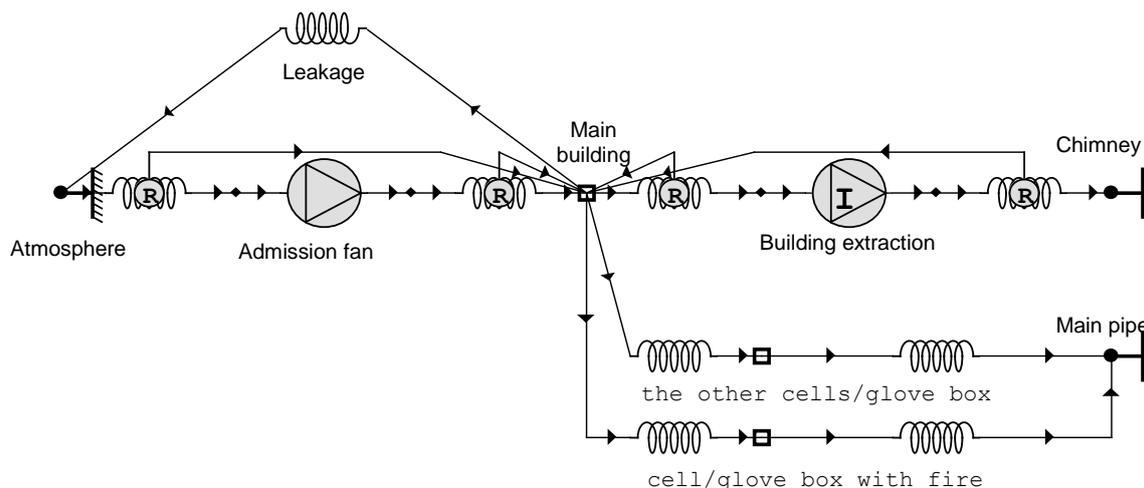
Figure 12: Ventilation schema and Sylvia impression of second scenario
