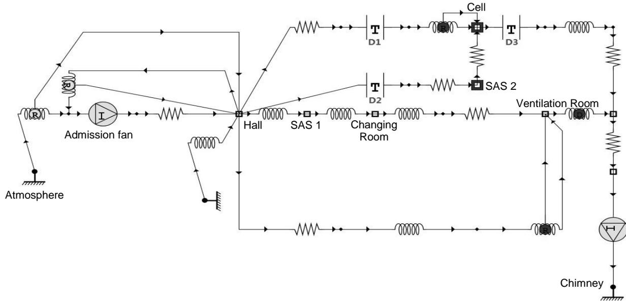
Figure 11: Ventilation schema and Sylvia impression of first scenario
