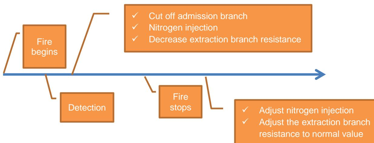
With this combined strategy, it could be observed that the hot cell never loses its underpressure. The gases temperature is never too high, which mean the filters are safe for temperature exposure (no analysis was made for water vapour in the smoke filters, which is one of the main reasons active carbon traps degrade). Also, the fire in the hot cell is
