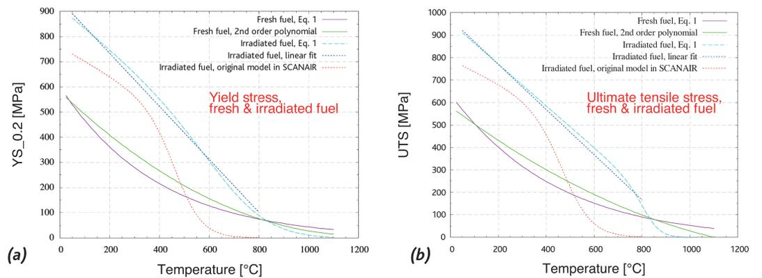
Fig 1 a-b: YS<sub>0.2</sub> (a) and UTS (b) of fresh and irradiated Zry-2.
